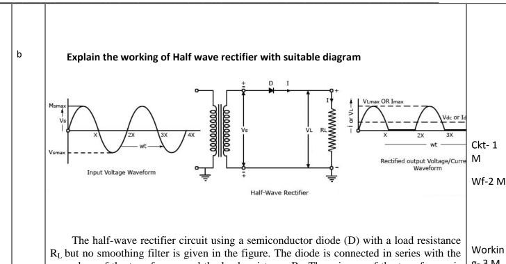
secondary of the transformer and the load resistance R<sub>L</sub>. The primary of the transformer is being connected to the ac supply mains.
